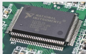
Single-chip IEEE 488.2 Talker/Listener interface to the GPIB
